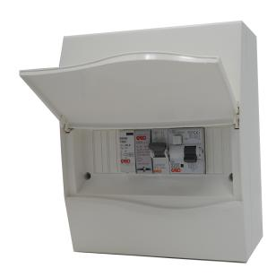
Garo Shower Boards are designed to facilitate the use of two electric showers which are being supplied from a domestic 63A single phase supply. Both showers may continually use <3kW of power each, however, when one exceeds this power use the Board will automatically cut the power to the second shower thus protecting the main supply fuse.
